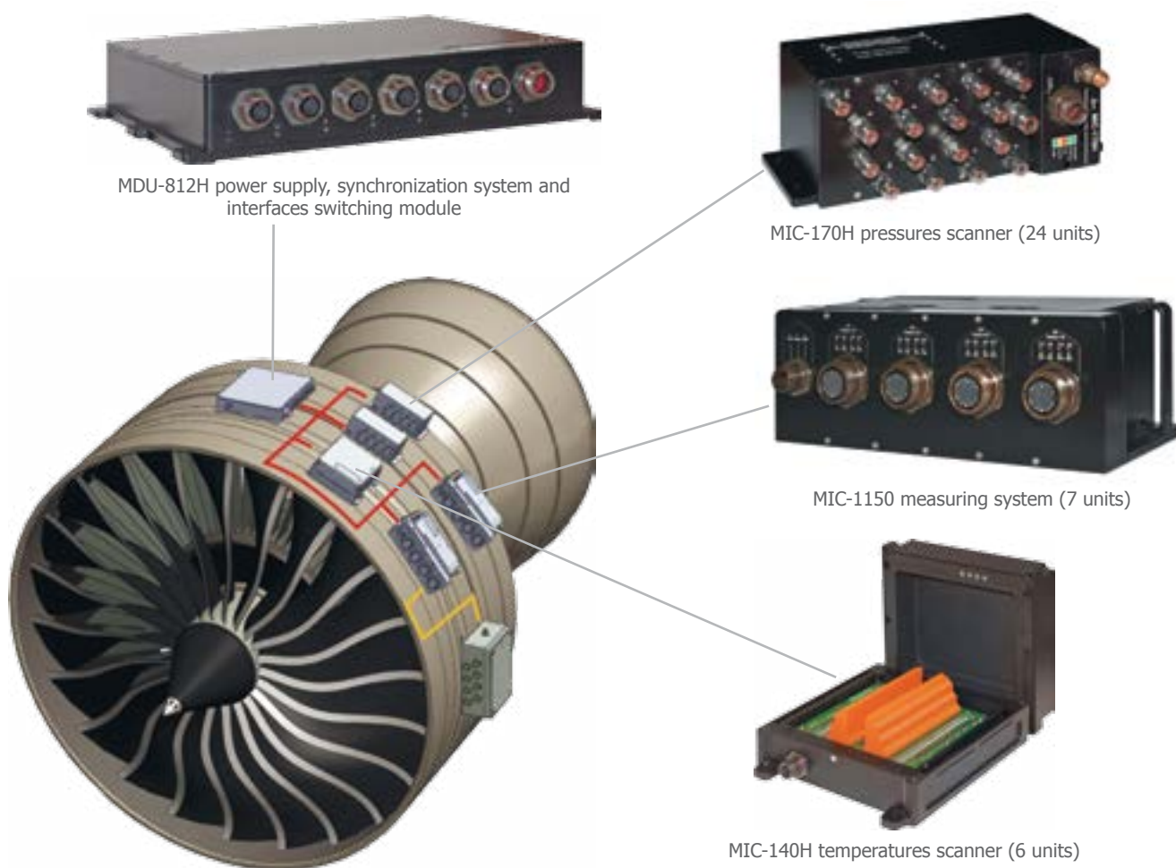
Placement of «Parus-LL» hardware on the aircraft engine
