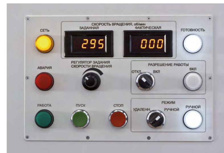
Control system for rotation platform of test-bench
