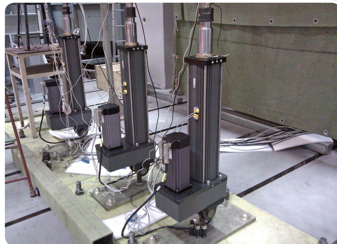
Electromechanical force actuators of loading system
